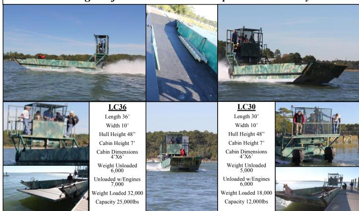
The Captain's Cockpit is raised above the deck of the *Landing Craft* for greater visibility. Manufactured with 3/16" aluminum. Featuring a hydraulic ramp in the front for loading vehicles and equipment from the shoreline. Custom sizes available. *Contains flotation foam within its hull.*
