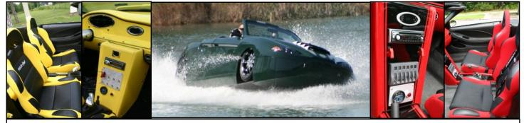
The Hydra Spyder is powered by a Corvette LS engine. 5 speed manual high performance close ratio transmission. Front wheel drive. The suspension system is air ride with retracting wheels and planing doors for high speed water usage.
