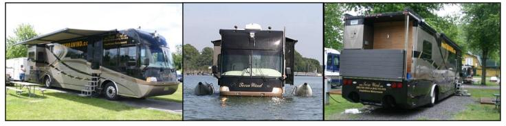
The Terra Wind was designed and created to have the outward appearance of a luxurious motor coach. It is not until the two (2) 19" bronze propellers are seen on the back of the vehicle that one realizes it is also a yacht.
