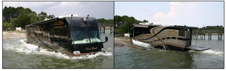
The Terra Wind is a beautiful, first class motor coach that doubles as a yacht. It can drive on the highway at speeds up to 80 mph. While on the water it can cruise at speeds up to 7 knots.
