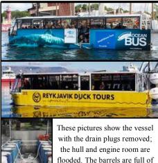
with the drain plugs removed; the hull and engine room are flooded. The barrels are full of water, equaling the weight as if fully loaded. The positive buoyancy assures the safety of the passengers.
