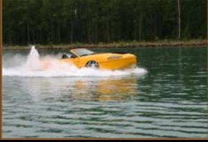
The standard production model Hydra Spyder is powered by a Corvette LS2 6.0-liter V8 engine rated @ 400 h.p. @ 6000 rpm and 400 ft. lbs of torque @ 4000 rpm. 5 speed manual high performance close ratio transmission. Front wheel drive with 3.73-1 axle ratio.
