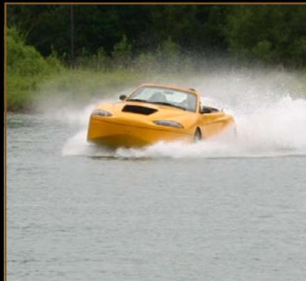
**Vehicle type:** front-engine, front-wheel drive, 4-passenger, 2-door, convertible top. Engine type: Corvette LS2 6.0-liter V8 engine.
